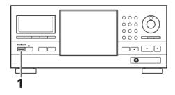
1 Press ტ **STANDBY/ON** on the front panel (එ on the remote control).
